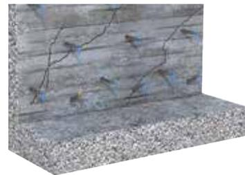
**3.** Fix the button head (non-return) fittings on the first packer and start the injection process at the lowest row of drill holes.
